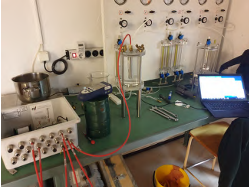
Figure C.16: Pressure cell for verification of calibration factors for VW piezometer sensors.
