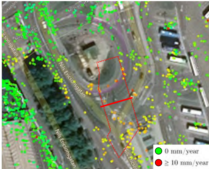
Figure C.4: Rate of on-going settlement in the area. Courtesy of Trafikverket. The sheet pile walls and the instrumented section are outlined in red.
