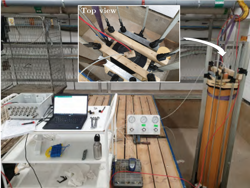
Figure C.18: Pressure cell for verification of calibration factors for VW total earth pressure sensors. The cell was assembled using clamps, since it had to be disassembled and reassembled for mounting of each of the total pressure cells (10 in total; 6 installed under the slab plus 4 additional which were decided to not install).
